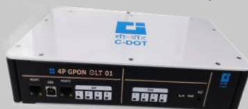
4 port Office OLT
