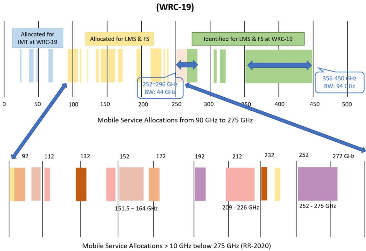
Figure 9: Spectrum above 30 GHz allocated to MOBILE services as per Radio Regulations (source: IAFI)
